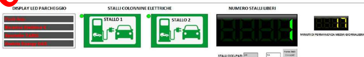
Figure 39 Real-Time Display Interface for Parking and EV Charging Management.
