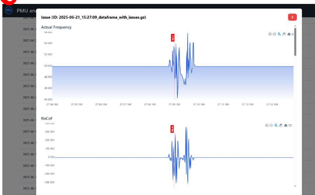
Figure 35 PMU analyzer issue visualization showing frequency and current magnitude anomalies in SE_01
